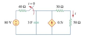
Q5: In the circuit shown below, find  $i_0$ ,  $v_0$  and i(t) for all time, assuming the switch was open for a long time. Also sketch i(t) and  $i_0$  on a same graph. [10]
