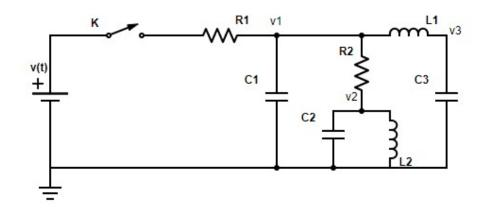
Q8: The network below reaches a steady state with the switch K open. At t = 0, switch K is closed. Find *i*(t) for the numerical values given, sketch the current waveform, and indicate the value of the time constant. [10]
