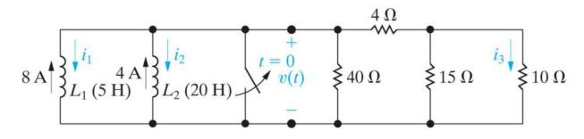
Q4: The switch is closed for long time and opened at t=0. Find  $i(0^{-})$  and i(t) and for t>0. [10]
