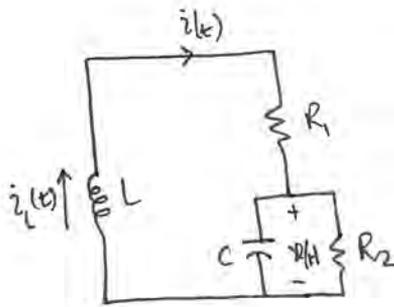
$$R_1 = 10\Omega ; R_2 = 8\Omega ; C = \frac{1}{8}F ;$$
