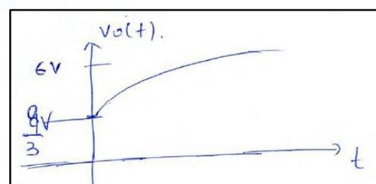
$$v_o(t) = K_1 + K_2 e^{-t/\tau}, \quad K_1 = v_o(\infty) = 6V, \quad K_2 = v_o(0^+) - v_o(\infty) = \frac{10}{3}V$$
