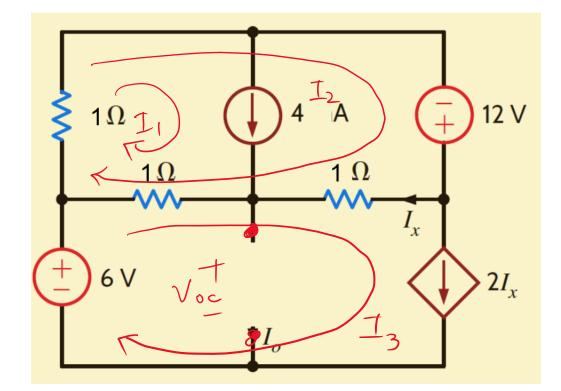
$$\begin{split} I_{1} = 4A, \quad I_{3} = 2I_{x} \\ \underline{Loop 2} = -12 + 1(I_{2} - I_{3}) + 1(I_{1} + I_{2} - I_{3}) \\ + (I_{1} + I_{2}) 1 = 0 \\ \underline{I}_{x} = I_{2} - I_{3} \implies 3I_{x} = I_{2} \\ \underline{I}_{3} = \frac{gA}{5}, \quad I_{2} = \frac{12}{5}A_{2} \quad I_{x} = \frac{4}{5}A \\ \nabla_{oc} = 6 + (I_{1} + I_{2} - I_{3}) 1 = \frac{54}{5}V \end{split}$$
