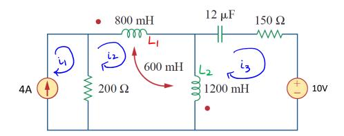
(a) (5 pts) Formulate the network equations using loop analysis.
