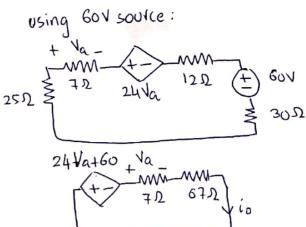
+ sinceflow of corrent is from negabive to positive in the 7.2 resistor, Va will be negative
