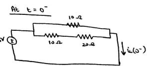
IN saturated inductor = short circuit
