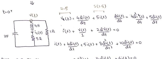
$$4\frac{di(d)}{d4} = 7.5 - 5(1.5) \qquad 8\frac{d^{2}i(t)}{d4} + \frac{14\frac{di(4)}{d4}}{d4} + 6i(4) = 0$$
