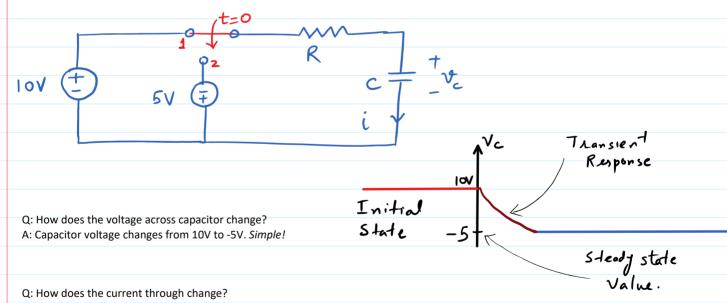
A: Current will be negative for some time and becomes zero (once capacitor voltage reaches -5V). Simple!
