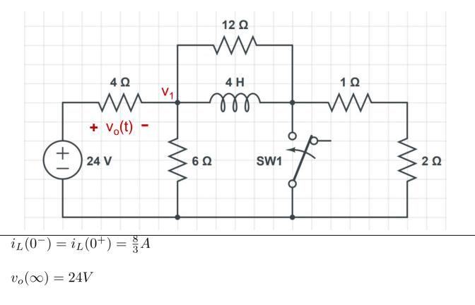
To find out i(0+), we use KCL to find  $v_1$  considering the bottom node as ground: (equation of the circuit at  $t = 0^+$ )
