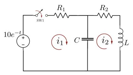
(a) (8 pts) Formulate the loop equations and eliminate  $i_1(t)$  to obtain a second-order differential equation for  $i_2(t)$ .
