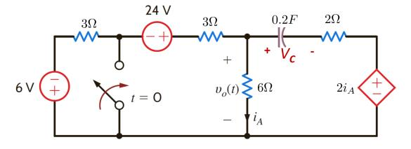
(a) (4 pts) Determine the voltage  $V_c(t)$  at  $t = 0^-$ , that is, just before the switch is operated.
