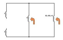
The arrowed inductors are parallel to eachother,
