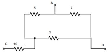
(b) The circuit is just a combination of parallel and series resistors
