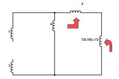
The arrowed inductors are in series
