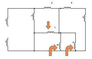
The arrowed inductors are in parallel since they share common nodes,
