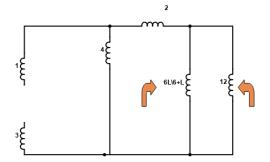
The two arrowed inductors are in parallel,
