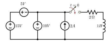
(b) (5 pts) For a circuit given below, assume that the switch is initially open and is closed at t = 0 and the inductor is not carrying any current before the switch is closed. Determine the voltage across the inductor and the total energy supplied to the inductor.
