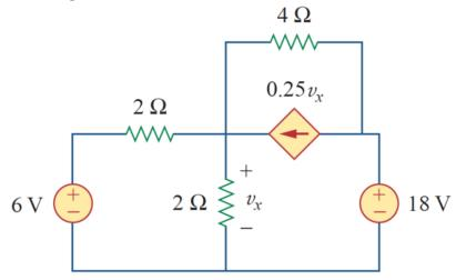
**Problem 9.** (12 pts) For the circuit given below, determine the current  $i_o$  using superposition principle. You can use any of the techniques (nodal analysis, loop analysis and source transformation) to carry out analysis when you keep one independent source in the circuit.
