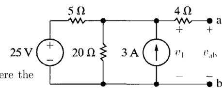
Taking bottom node as ground node and applying KCL at a node where the voltage is  $v_1$
