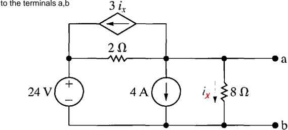
\* Circuit contains both dependent and Independent Sources; we can use either of the following techniques
