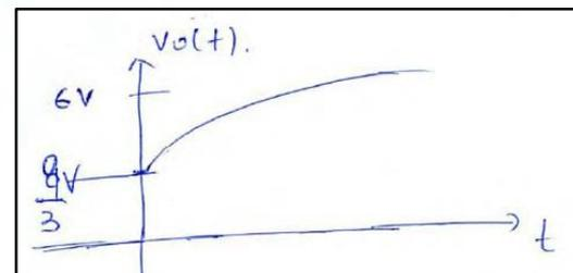
$$v_o(t) = K_1 + K_2 e^{-t/\tau}, \quad K_1 = v_o(\infty) = 6V, \quad K_2 = v_o(0^+) - v_o(\infty) = \frac{10}{3}V$$
