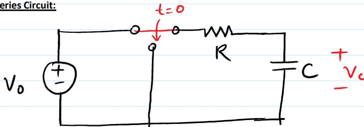
Problem 1: Determine the voltage across capacitor for  $t \geq 0$ .
