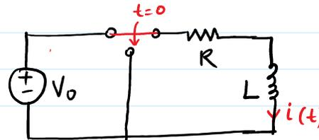
Initial conditions (state) of the inductor (Analyse circuit at  $t=0^-$ )
