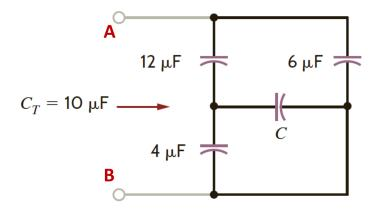
**Solution:** We have  $4\mu$  and C are in parallel and their parallel combination is in series with  $12\mu$ , that is,  $(4+C)12\mu/(4+C+12)$ . Let  $C_1=(4+C)12\mu/(4+C+12)$ . This equivalent capacitor  $C_1$  is in parallel with  $6\mu$  and therefore  $6+C_1=10\mu$ , which implies  $C_1=4\mu\,\mathrm{F}$  and  $C=2\mu\,\mathrm{F}$ .
