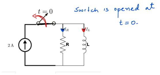
(b) (6 pts) Plot the waveforms (not to the scale but label the axes and indicate intercepts) of the currents  $i_R(t)$  and  $i_L(t)$ .
