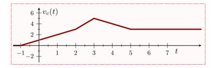
(c) (2 pts) Determine the energy stored in the capacitor at t = 3 seconds.  $w_c(t) = \frac{1}{2}C(v_c(t))^2 \Rightarrow w_c(3) = \frac{1}{2}(v_c(3))^2 = 12.5 J.$
