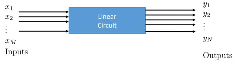
Each output  $y_k(t)$  is a linear combination of inputs and/or derivatives of inputs.
