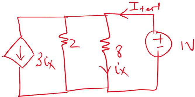
$$\Rightarrow R_{th} = \frac{1V}{I_{test}} = \boxed{1 \Omega}$$
