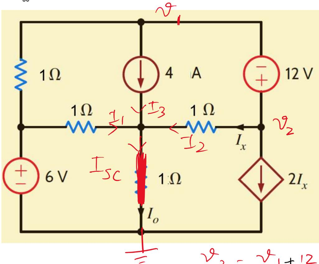
$$v_2 = v_1 + 12 \text{ (Super Node)}$$
