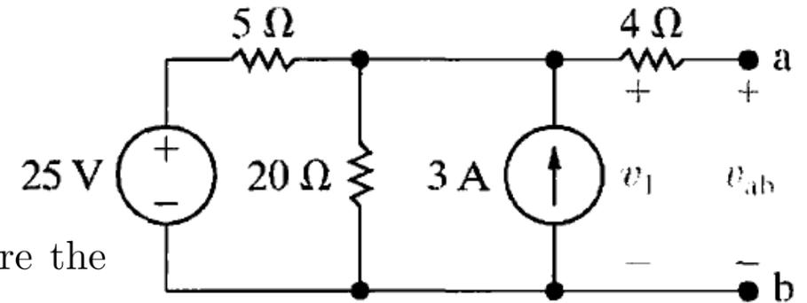
Taking bottom node as ground node and applying KCL at a node where the voltage is  $v_1$
