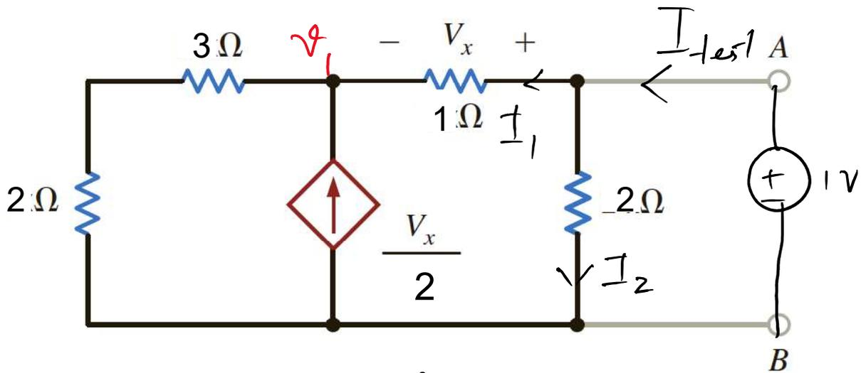
$$\frac{v_1}{5} + \frac{v_1 - 1}{1} = \frac{v_x}{2} \quad \left\{ \begin{array}{l} v_x + v_1 = 1 \\ \Rightarrow v_x = 1 - v_1 \end{array} \right.$$
