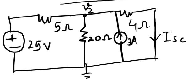
$$-3 + \frac{v_2 - 25}{5} + \frac{v_2}{20} + \frac{v_2}{4} = 0$$
