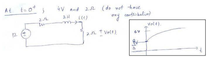
$v_o(t) = K_1 + K_2 e^{-t/\tau}, \quad K_1 = v_o(\infty) = 6V, \quad K_2 = v_o(0^+) - v_o(\infty) = \frac{10}{3}V$
