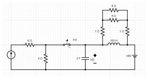
Q1) The circuit contains a 2A current source. The switch is opened at t=0.
