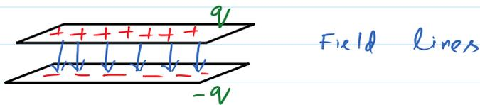
Capacitors in uncharged state do not carry any charge. During the charging phase, charge moves from one conductor to the other; making one conductor positively charged and other negatively charged (net charge on the capacitor is zero).
