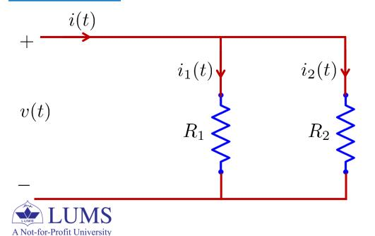
$$i_1(t) = \frac{R_2}{R_1 + R_2} i(t)$$
