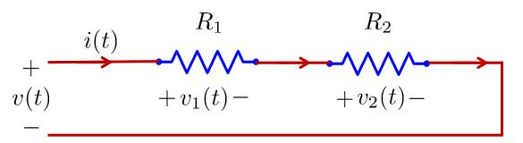
$$v_1(t) = \frac{R_1}{R_1 + R_2} v(t)$$
