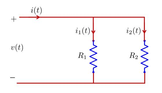
$$i_{1}(t) = \frac{v(t)}{R_{1}}, \quad i_{2} = \frac{v(t)}{R_{2}}$$
