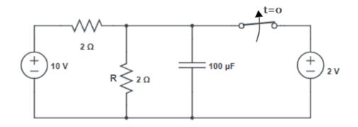
(b) [20 marks] Calculate i(t) for all t using Step by Step Analysis technique.
