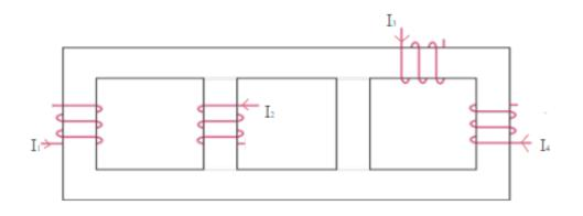
(b) [15 marks] For the circuit given below, apply Loop Analysis to obtain the complete set of loop equations. Make sure to adhere to the dot convention.
