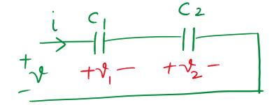
Same current (-> same charge => i <> q  $v_1 = \frac{q}{c_1}$ ,  $v_2 = \frac{q}{c_2}$  =>  $v = q(\frac{1}{c_1} + \frac{1}{c_2})$   $v = \frac{q}{c_1}$ ,  $v_1 = \frac{1}{c_2}$ ,  $v_2 = \frac{q}{c_2}$  =>  $v = q(\frac{1}{c_1} + \frac{1}{c_2})$   $v = \frac{q}{c_1}$ ,  $v_2 = \frac{1}{c_2}$ ,  $v = q = \frac{1}{c_1}$
