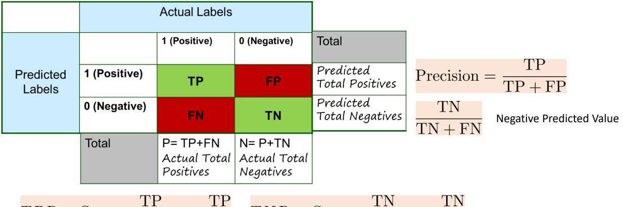
$$TPR = S_e = \frac{11}{\text{TP} + \text{FN}} = \frac{11}{\text{P}} \quad TNR = S_p = \frac{11}{\text{TN} + \text{FP}} = \frac{11}{\text{N}}$$
