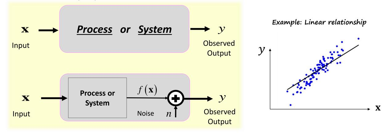
Here, PROCESS or SYSTEM refers to any underlying physical or logical phenomenon which maps our input data to our observed and noisy output data.
