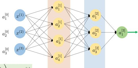
$$\frac{\partial \mathcal{L}}{\partial \mathbf{z}^{[1]}} = \left( \mathbf{W}^{[2]^T} \frac{\partial \mathcal{L}}{\partial \mathbf{z}^{[2]}} \right) \odot g'(\mathbf{z}^{[1]}) = \left( \mathbf{W}^{[2]^T} \left( \left( \mathbf{W}^{[3]^T} \frac{\partial \mathcal{L}}{\partial \mathbf{z}^{[3]}} \right) \odot g'(\mathbf{z}^{[2]}) \right) \odot g'(\mathbf{z}^{[1]})$$
