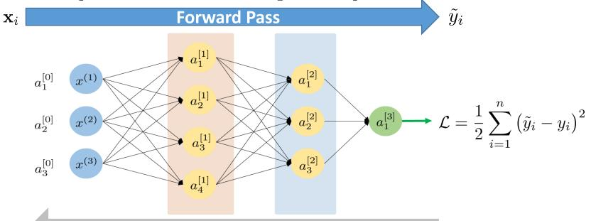
The weights are the only parameters that can be modified to make the loss function as low as possible.
