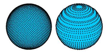
Fig. 2: Visual comparison of sampling density between HEALPix and proposed sampling scheme for bandlimit, L=32.
