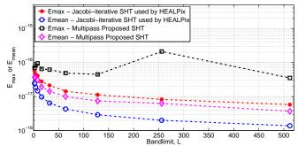
Fig. 3:  $E_{\rm max}$  and  $E_{\rm mean}$  between spectral coefficients of the original and reconstructed signals for band-limits in the range 2 < L < 512.
